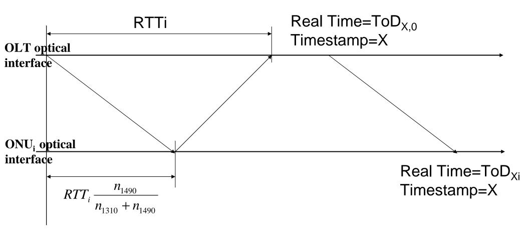
$$RTT_i = T_{\text{downstream}} + T_{\text{upstream}}$$
