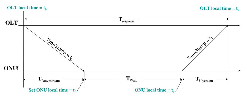
$T_{\text{downstream}} = \text{downstream}$  propagation delay
