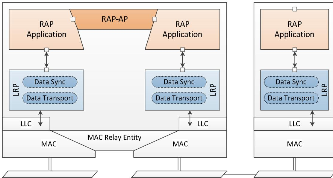
Figure 2 - Architecture of RAP on a Bridge and an end station
