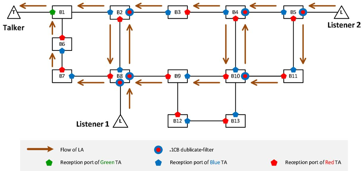
Figure 10 - RAP Listener attribute propagation for ladder redundancy
