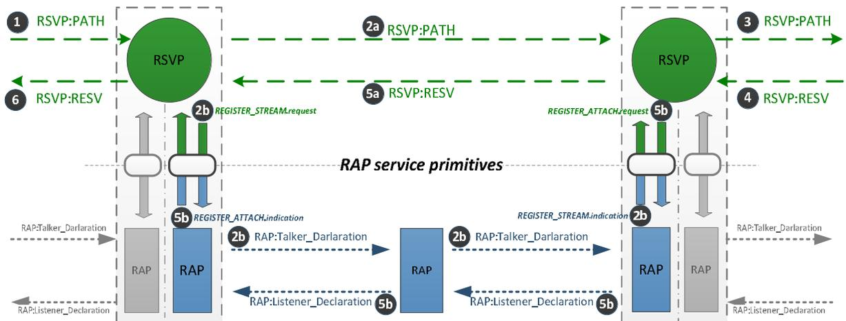
Figure 12 – Parallel operation of RSVP and RAP within a L2 sub-network
