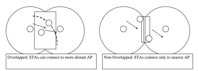
Figure 2 - Overlapped and Non-Overlapped BSA Coverage
