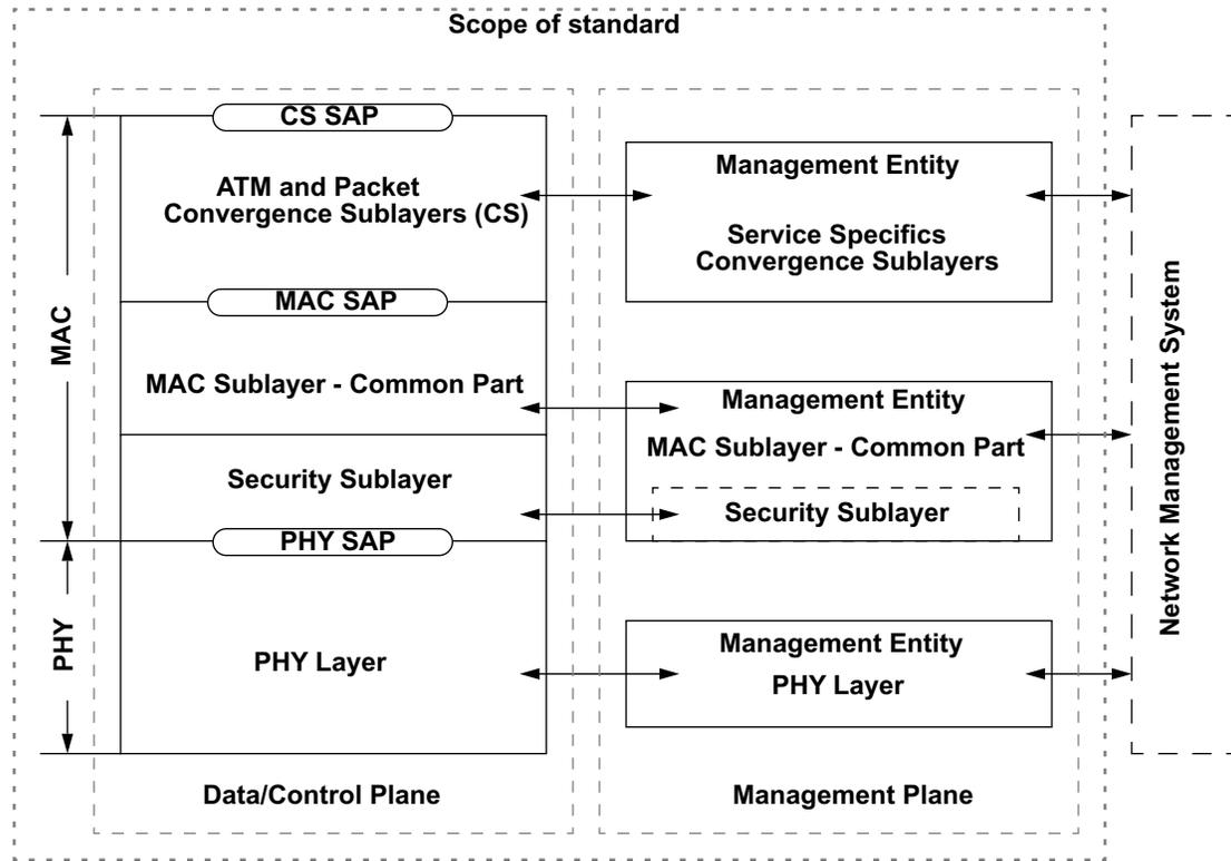
FIGURE 1. IEEE 802.16 Reference Model and Protocol Stack
