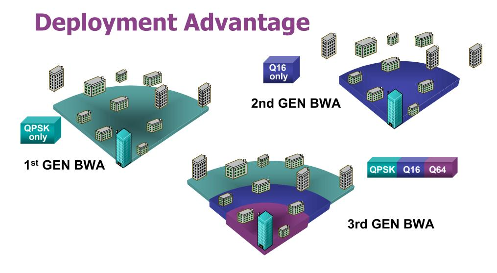
More than 2x Capacity & 2x Coverage with Adaptive Modulation
