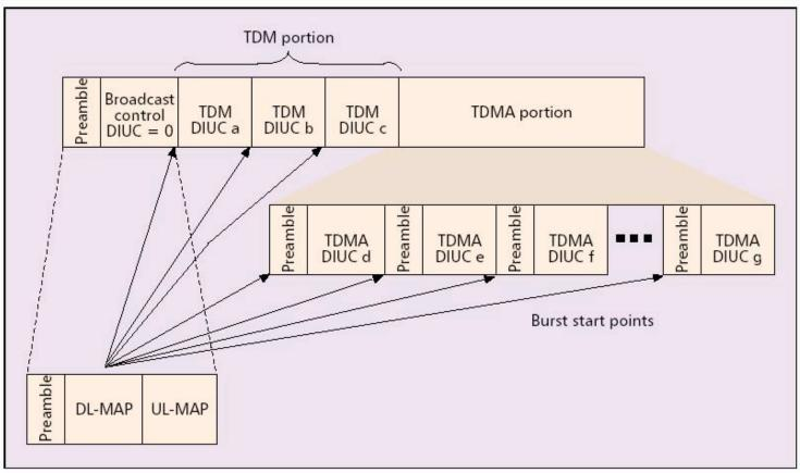
TDMA portion: transmits data to some half-duplex SSs (the ones scheduled to transmit earlier in the frame than they receive)
