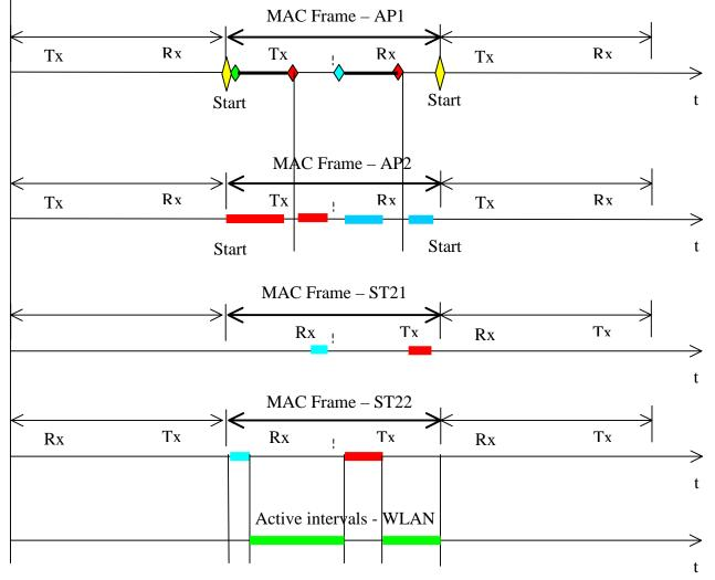
Figure 3 Communications intervals when applying sharing protocol
