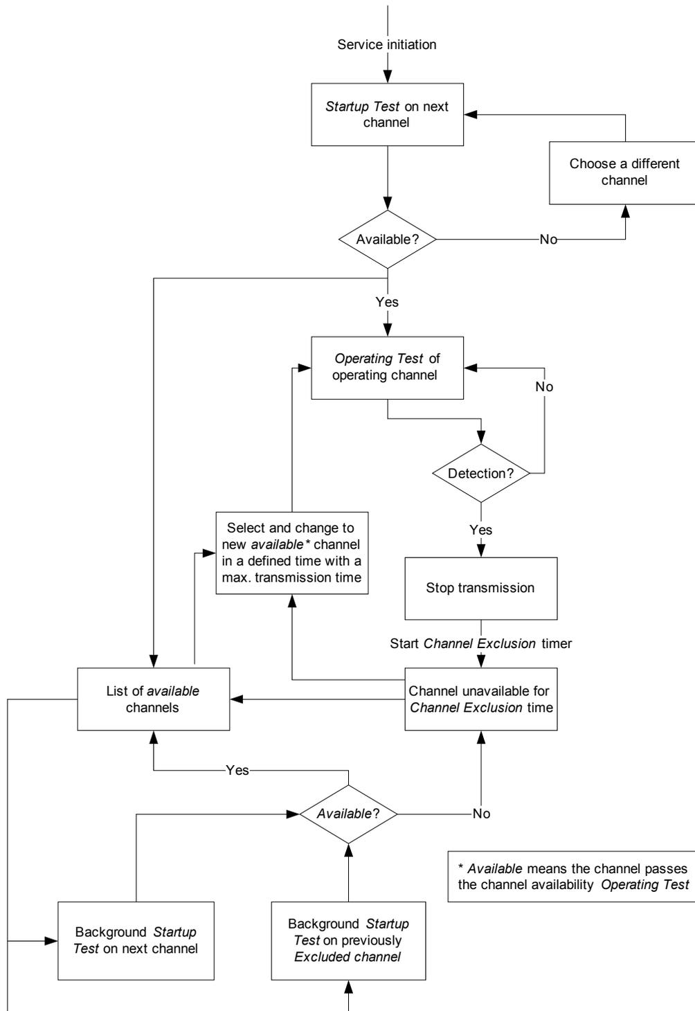
Figure 1 Flowchart algorithm for specific spectrum users.
