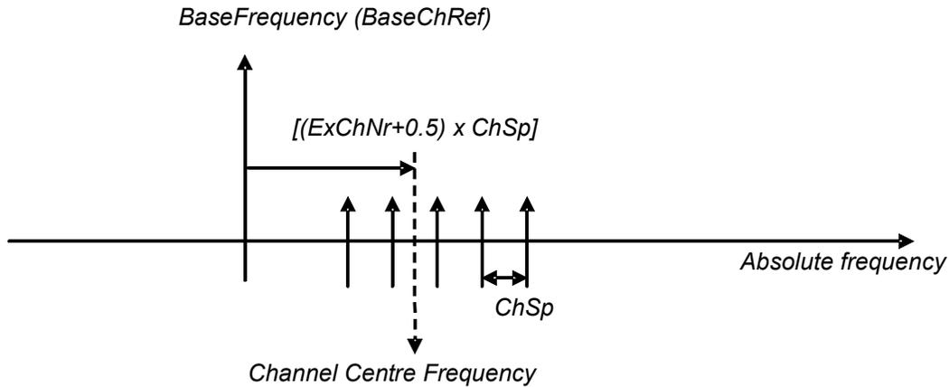
**Figure 2** Representation of extended channel numbering structure.
