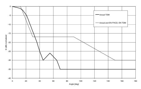
Figure A2: Antenna pattern envelope on the azimuth plane.
