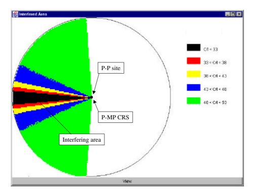
Figure B14: Cell area of potential sources (TS) of interference (class B3) and their relevant C/I generated on the P-P receiver.
