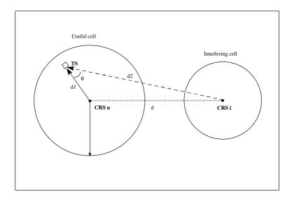
Figure 6.2: Generic scenario for class A1 interference analysis.
