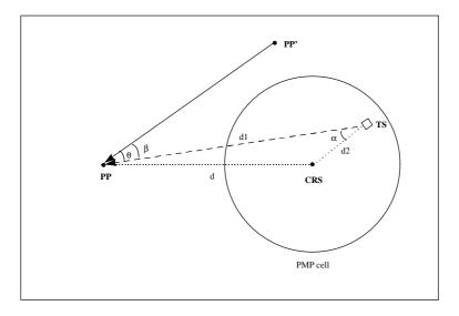
Figure 7.3: Generic scenario for class B3 interference analysis.
