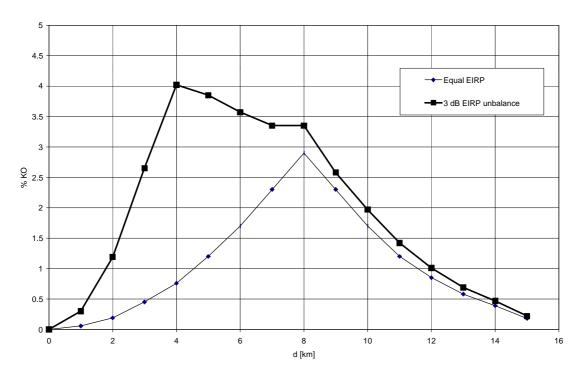
Figure A3: %KO area for class A2 (TDM on FHCD) with ETSI limits.
