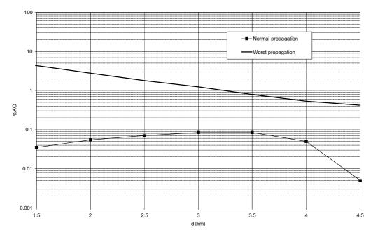
Figure A10: %KO area for FDM system (class A1, 28 MHz guard band).
