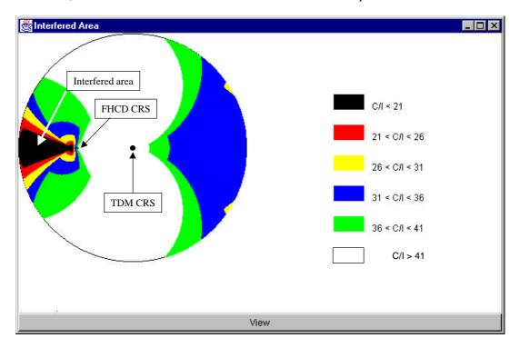
Figure A4: C/I distribution over the TDM cell area.
