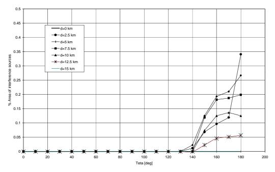
Figure B5: % of cell area for any potential TS interfering P-P (class B3).
