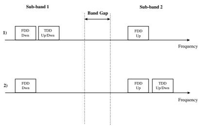
Figure 5.2: Possible arrangements for a FDD P-MP system and a TDD P-MP system
