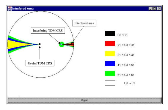
Figure A7: C/I distribution over the useful TDM cell area for CRS distance of 2 km.
