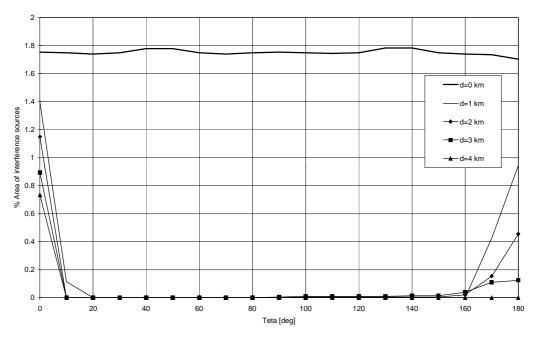
Figure B12: % of cell area for any potential TS interfering P-P (class B3).
