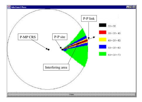
Figure B7: Cell area of potential sources (TS) of interference (class B3) and their relevant C/I generated on the P-P receiver.
