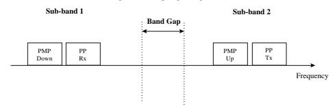
Figure 9.1: Useful channel arrangement.
