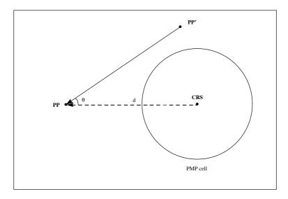
Figure 7.1: Generic scenario for class B1 interference analysis.
