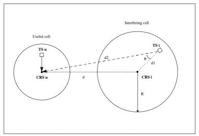
Figure 6.3: Generic scenario for class A2 interference analysis.
