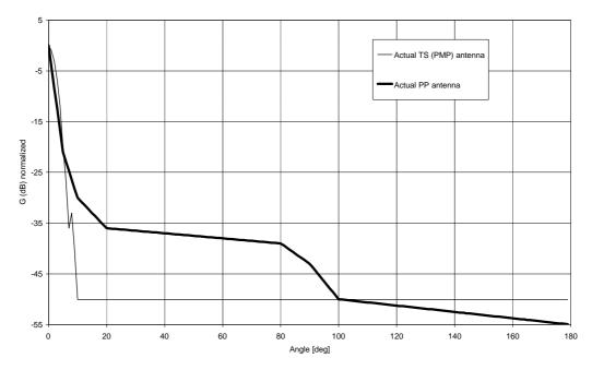
Figure B9: Antenna pattern envelope on the azimuth plane.
