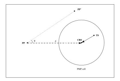
Figure 7.2: Generic scenario for class B2 interference analysis.
