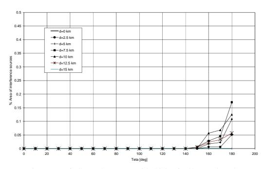
Figure B6: % of cell area where any potential TS is interfered by P-P (class B4).
