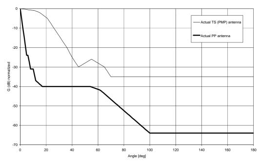
Figure B2: Antenna pattern envelope on the azimuth plane.
