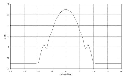
Figure A5: Antenna pattern envelope on the azimuth plane.
