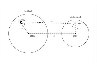
Figure 6.5: Generic scenario for class A4 interference analysis
