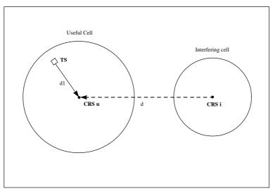
Figure 6.4: Generic scenario for class A3 interference analysis
