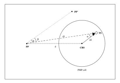
Figure 7.4: Generic scenario for class B4 interference analysis.
