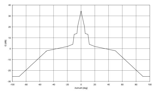
Figure A8: TS antenna pattern envelope, on the azimuth plane, for FDM system.
