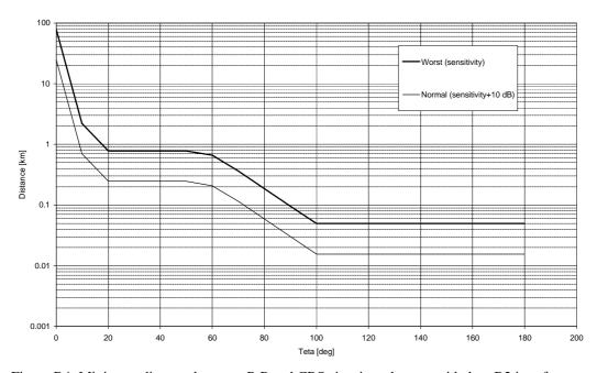
Figure B4: Minimum distance between P-P and CRS sites in order to avoid class B2 interference.
