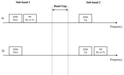
Figure 5.3: Possible arrangements for a FDD P-MP system and a P-P system
