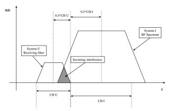
Figure 6.1: Adjacent channel interference behaviour.
