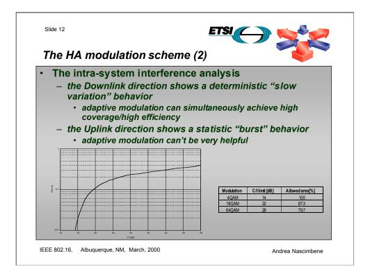
The C/I ratio in the downlink is a function of the position of the AT within the cell (or sector). Considering the reuse scheme with 2 frequencies and 2 polarisation, and a  $90^{\circ}$  sectored antenna the C/I distribution within a sector is the one reported in the above figure.
