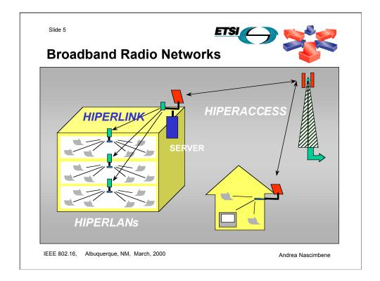
The figure shows an example of how the three network categories might be deployed in a business and domestic environment. In both cases, HIPERACCESS provides the means to reach the premises of the customer.
