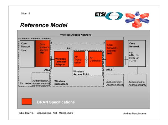
The high level reference model used by the project as basis for its cooperation with the ATMForum and ETSI SMG is shown in this picture which also shows the scope of the work of the project.
