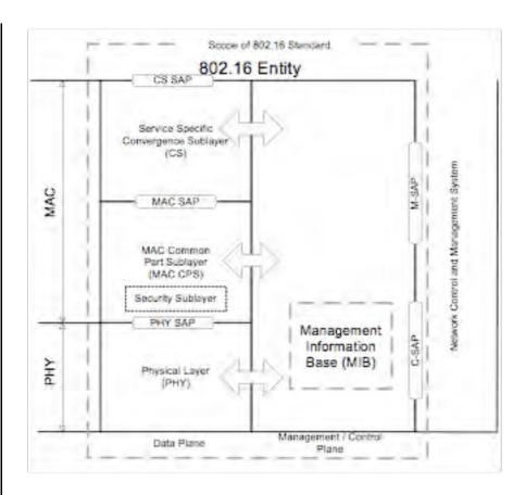
The MAC CPS provides the core MAC functionality of system access, bandwidth allocation, connection establishment, and connection maintenance. It receives data from the various CSs, through the MAC SAP, classified to particular MAC connections.
