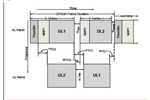
For systems that serve only F-FDD MSs, the frame structure is configured by allocating the whole down link and uplink frames to the F-FDD MSs without partitioning of frames.
