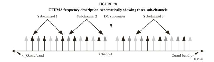
Sub-channelization is a multiple access technique. It provides OFDMA systems increased scheduling flexibility and a number of performance advantages, including enhanced scalability and advanced antenna array processing capabilities.
