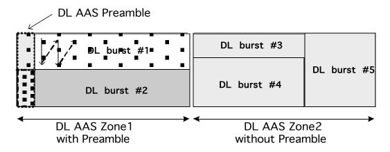
Fig. XXX. Burst Allocations in DL AAS Zone
