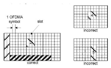
Figure 222a—Example of UIUC = 12,13 allocation rules
