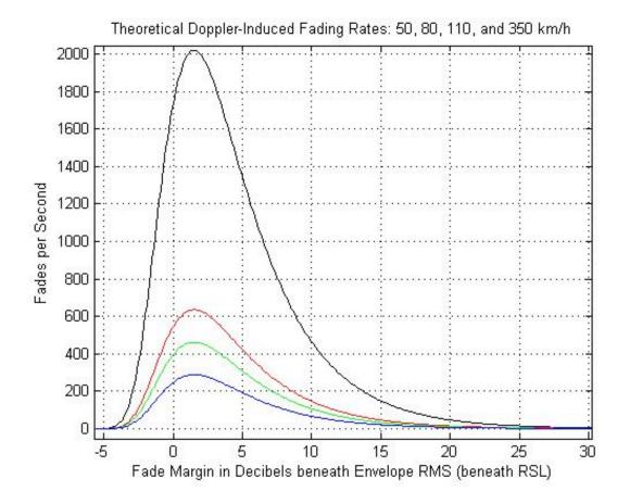
Figure 6-1. Number of Doppler induced fades per second for different speed rates.
