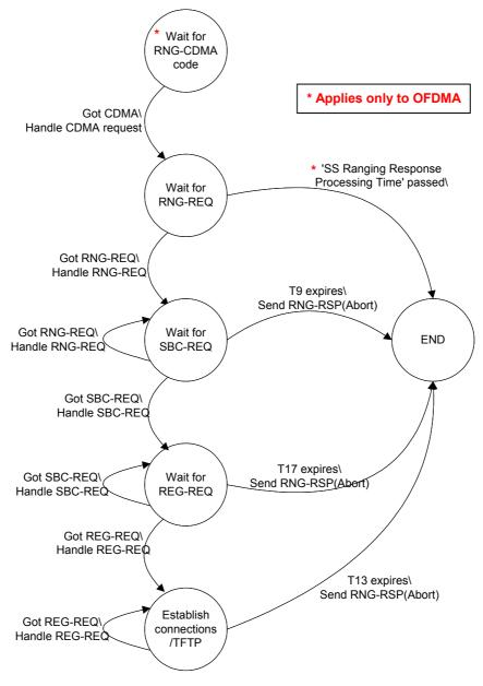
Figure 70a – Network entry state-machine BS side.
