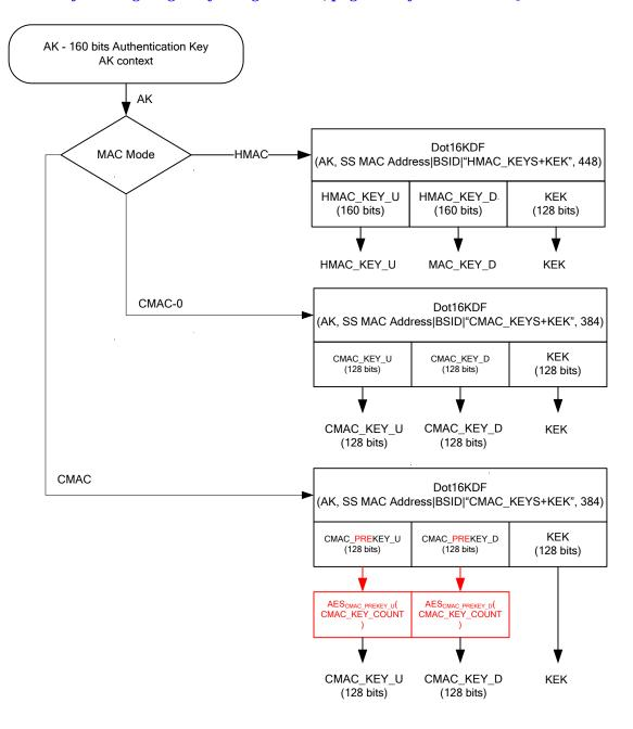
Figure 130o—HMAC/CMAC/KEK derivation from AK
