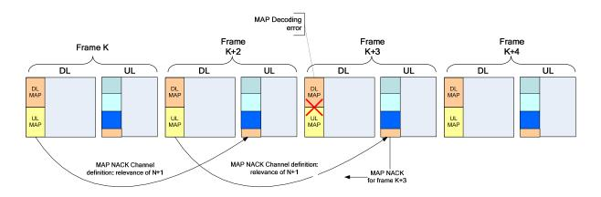
MAP ACK relevance is proposed to be N+1 to allow MS sufficient time to prepare the MAP ACK and to be consistent with HARQ ACK/NACK time. (The HARQ ACK/NACK time is determined by the HARQ ACK delay parameter.) This is illustrated in the figure below.
