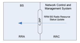
Figure 3: Example Primitive Flow of Radio Resource Status Update
