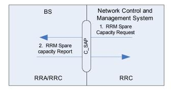
Figure 2: Example Primitive Flow of Spare capacity Report
