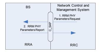
Figure 1: Example Primitive Flow of Physical Parameter Report
