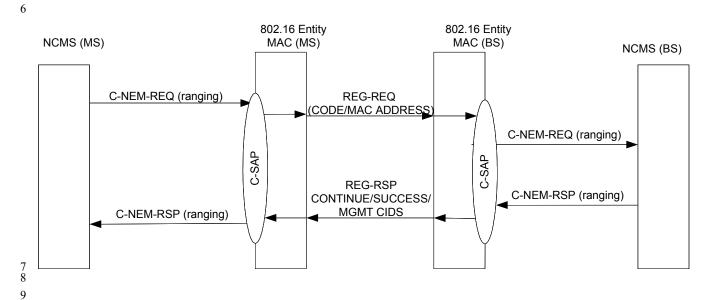
Figure 498 – Ranging Primitives (MS and BS)
