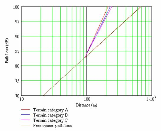
The result shows that the new breakpoint distance has the desired effect. It has now reduced for the path loss calculation at 3.5GHz.
