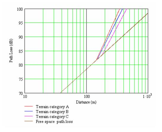
The corrected breakpoint increases with terminal antenna height, as expected.
