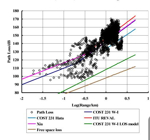
Comparison of 2GHz path loss measurements in Central London with several path loss models.
