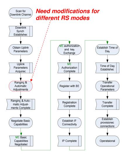
Figure 1: Network Entry Procedure for MS
