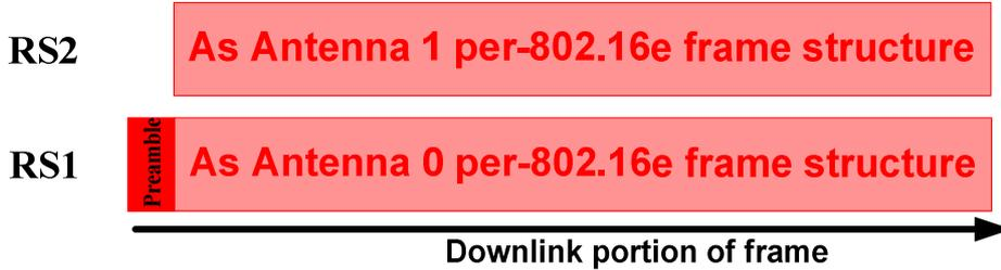
5- VBS made of BS and several RS, only BS transmits the preamble. In this case the MS regards the VBS as a BS with antenna array. The BS transmitting the preamble is antenna 0, and other RS are antenna 1, 2 and 3.
