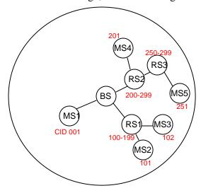
Figure 2 CID Assignment for Example 3.1
