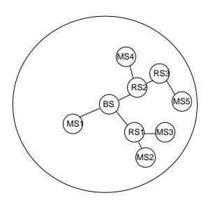
Figure 1 Relay System Topology Example
