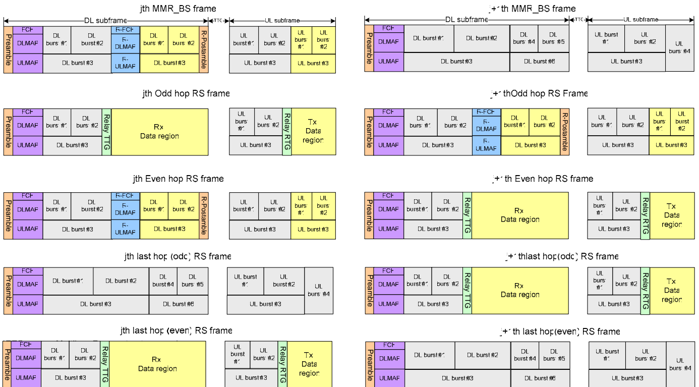
Figure B. An example of multi-hop relay environment showing a 3-hop relay
