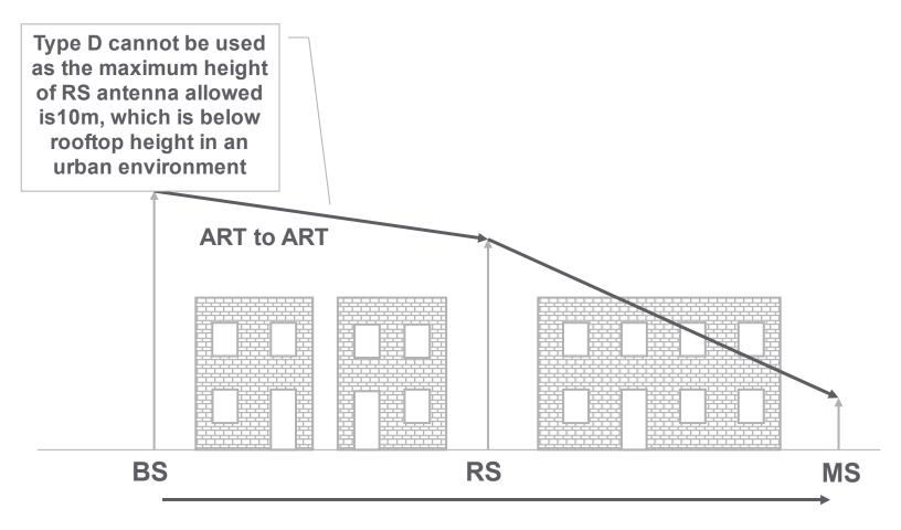
ART to BRT (NLOS) model (cost 231 Walfisch-Ikagami model) for urban includes several hops of over-the-building propagation component and a rooftop\_to\_street diffraction (last hop) component. 3
