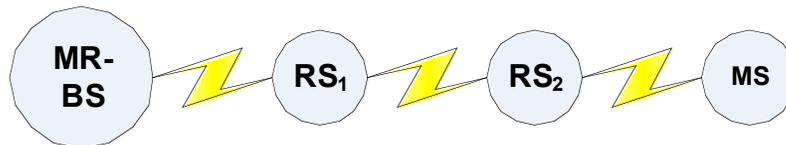
**Figure 1: Example Topology in multi-hop relay System**
