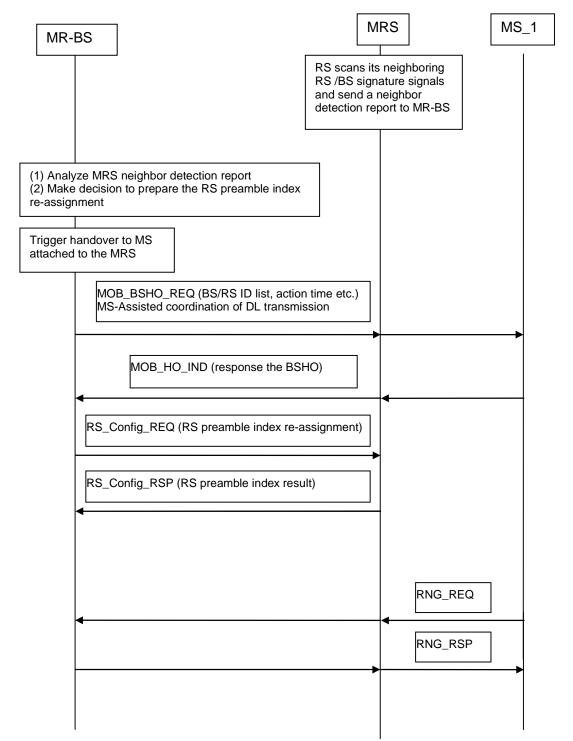
Figure 1. The message signaling for the mobile RS preamble segment re-assignment.
