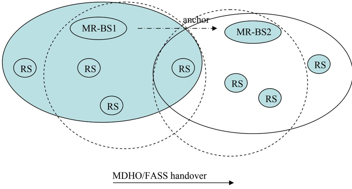
Figure 6 : Inter MR-BS handover, the current anchor station and target anchor station is the different MR-BSs
