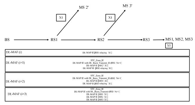
Figure 2a Example of proposed MAP-based scheme for multicast data relaying (one hop in one frame)
