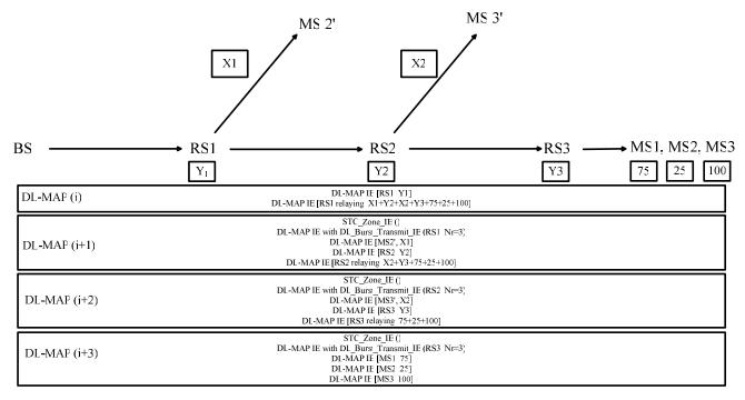
Figure 1a Example of proposed MAP-based scheme for unicast data relaying (one hop in one frame)
