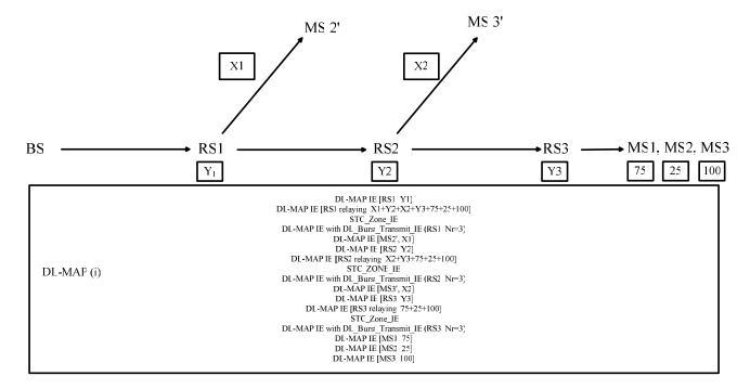
Figure 1b Example of proposed MAP-based scheme for unicast data relaying (all hops in one frame)
