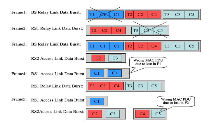
Figure 2. Example of MAC PDU relay
