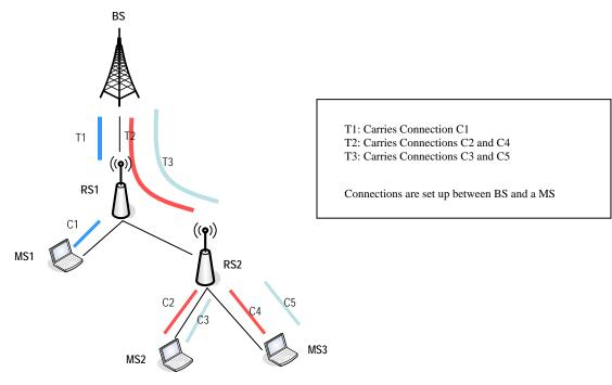
Figure 1 Example of 3 hops Relay
