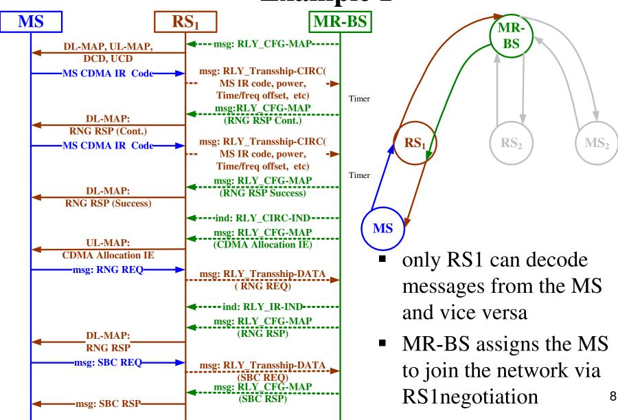
MS joining Multihop Relay Network via RS
