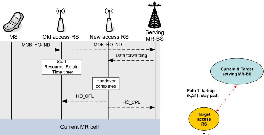
\*This flow is an example when a direct 1-hop relay link exists between the current and the target access RSs.
