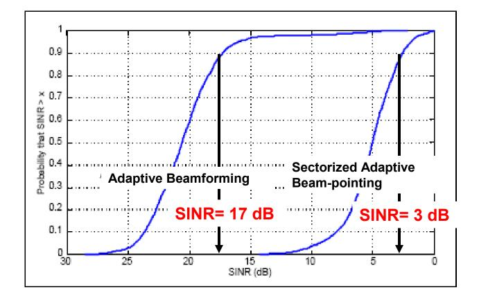
Adequate SINR for 10 Simultaneous Link at <sup>3</sup>/<sub>4</sub> rate 64 QAM
