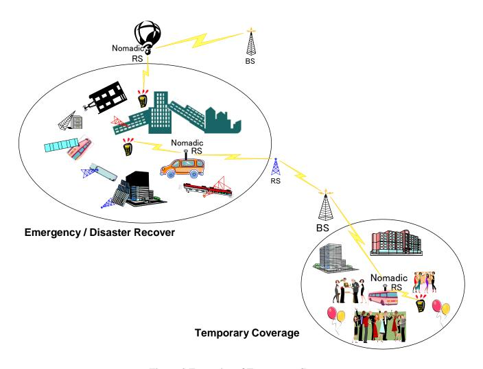
Figure 3 Examples of Temporary Coverage
