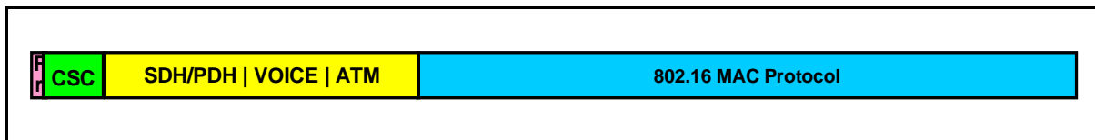
Figure N-2. Example of Element Address (logical) domain assignments for supporting 802.16 MAC, SDH/PDH, Voice and ATM Channels
