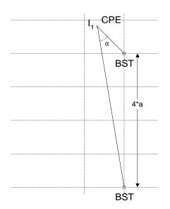
The triangle created by the interfering CPE, its BST, and the interfered BST a known angle. The angle a represents half the beam width of the CPE antenna. Known is also the distance between the BST units, that is four times the cell width, a. Using some geometric identities we can express the x-y coordinates of the interference boundary curve in parametric form (h is the parameter),
