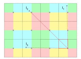
We will use a geometric analysis to try to determine what is the percentage of CPE units that might cause interference to a neighboring cell. The drawing below shows what are the geometric relations a CPE unit in cell  $I_1$  is required to fulfill in order to be considered a source of interference.
