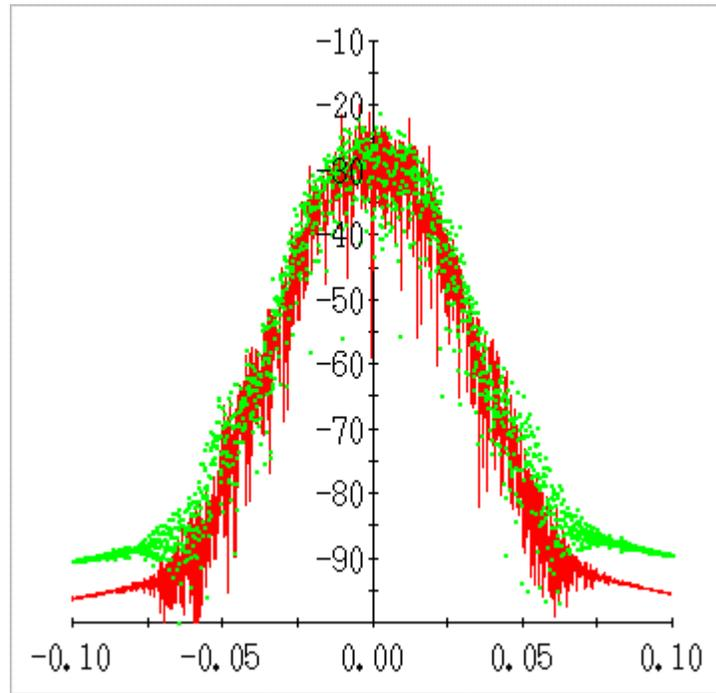
Figure 6. The modulated spectra of GMSK with BT = 0.22 and CQPSK overlaid for comparison. The GMSK signal is represented with green points, while the CPQSK signal is indicated by the red lines. Spectral occupancy of the two modulations is essentially the same.
