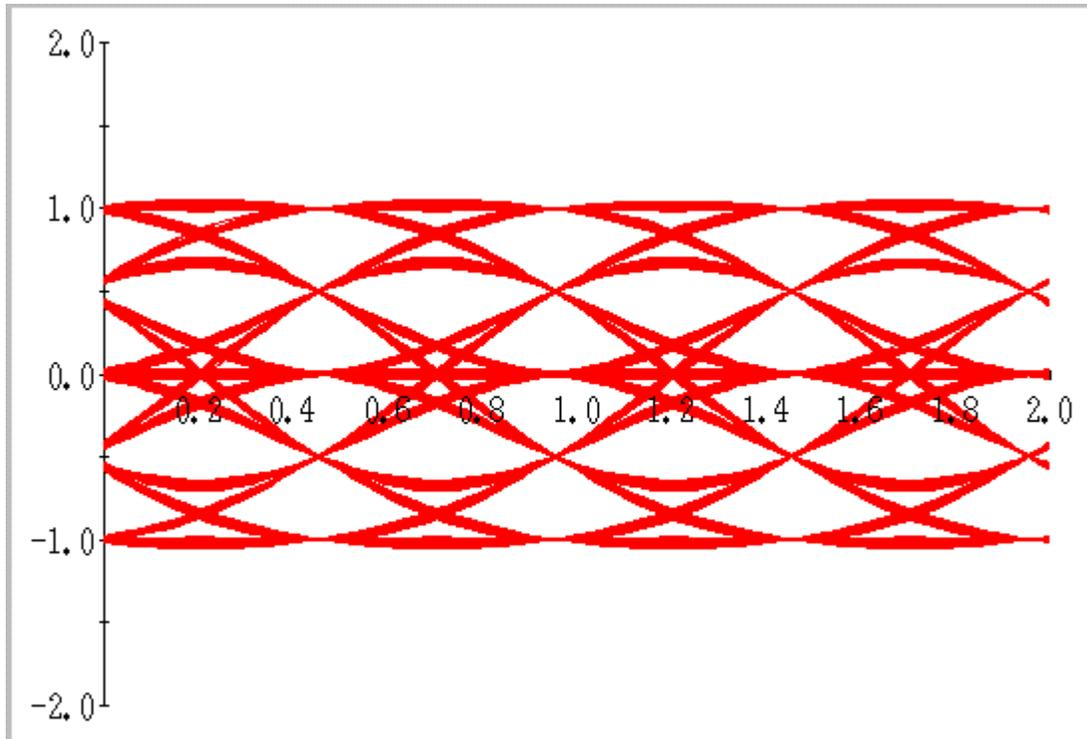
Figure 3. Four symbols of CQPSK filtered phase.
