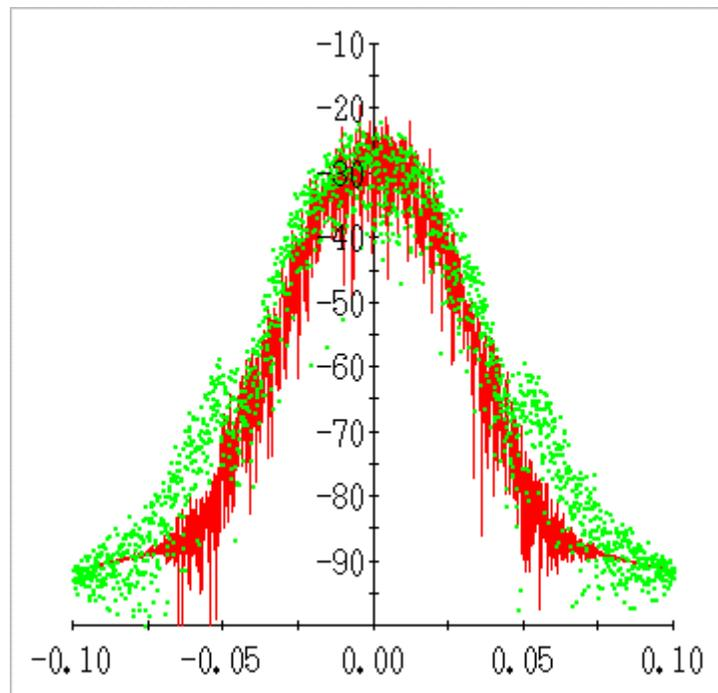
Figure 5. The modulated spectra of GMSK with  $BT = 0.3$  and CQPSK overlaid for comparison. The GMSK signal is represented with green points, while the CQPSK signal is indicated by the red lines. Since the modulated symbols are each 32 samples long in the simulation, the symbol rate range is  $\pm 0.015625$  in the horizontal scale.
