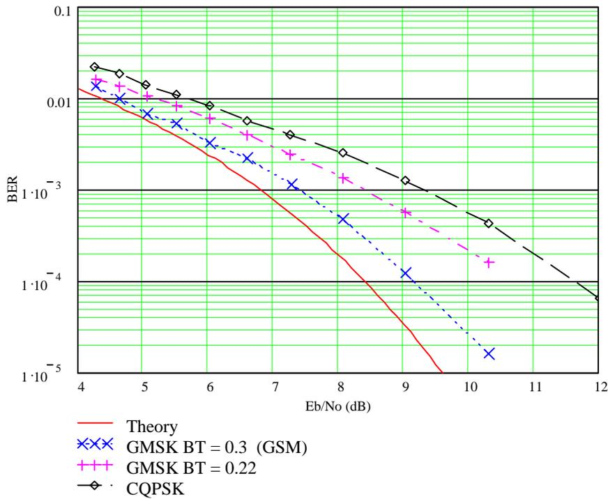
Figure 7. BER for coherent reception of GMSK and CQPSK in AWGN.
