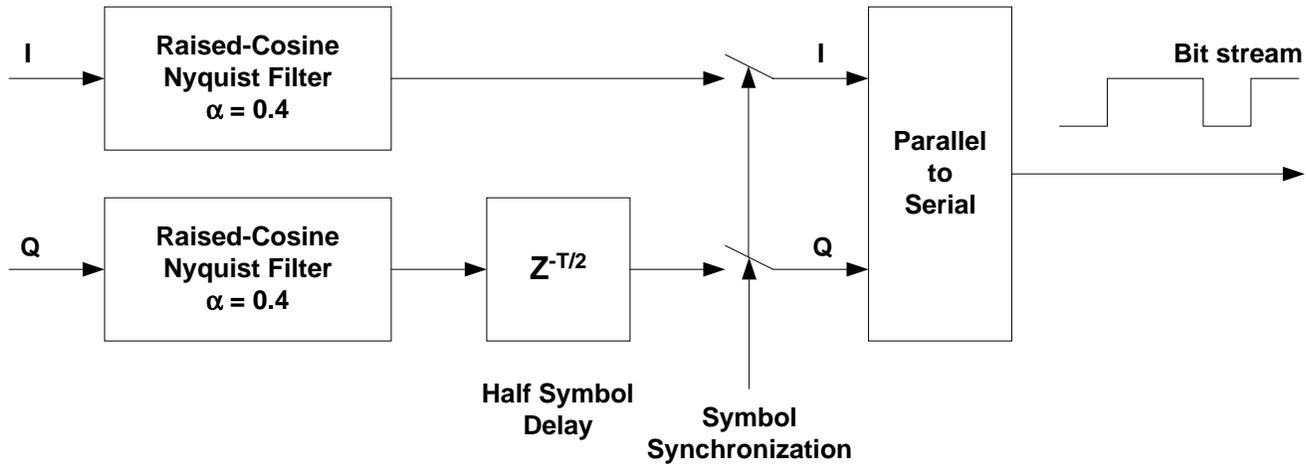
Figure 4. Block diagram of simulation demodulator model.
