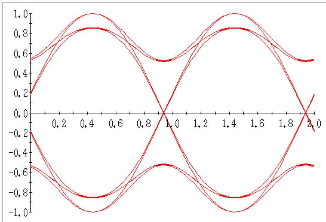
Figure 10. Modulator Eye Diagram for GMSK with  $BT = 0.3$ . The ISI is exhibited in the additional level in the peak region.
