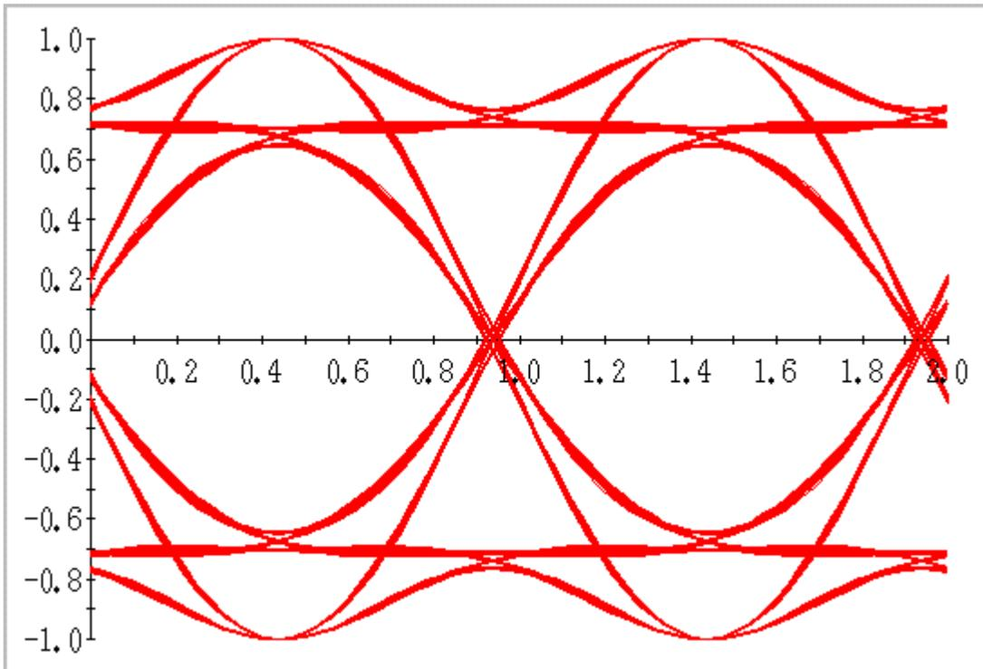
Figure 11. Modulator Eye Diagram for CQPSK. The additional ISI in comparison to the GMSK signal is clear.
