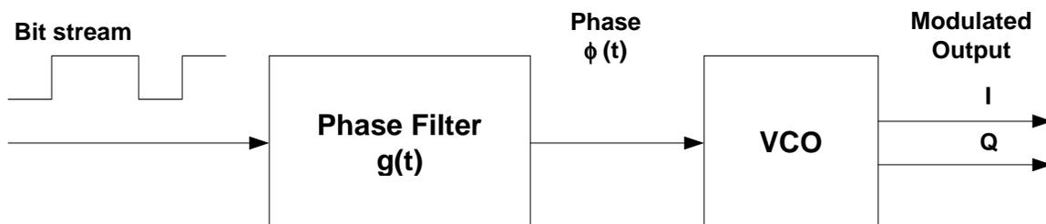
Figure 1. Basic Phase Modulator with Phase Filter.
