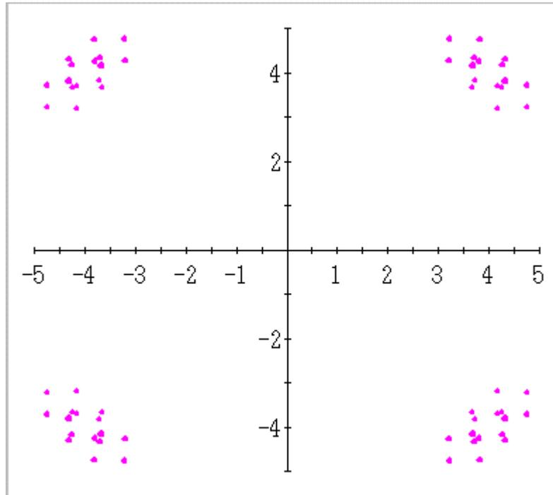
Figure 8. GMSK receive constellation for  $BT = 0.3$ . The ISI due to the gaussian phase filter spreads the four constellation points.
