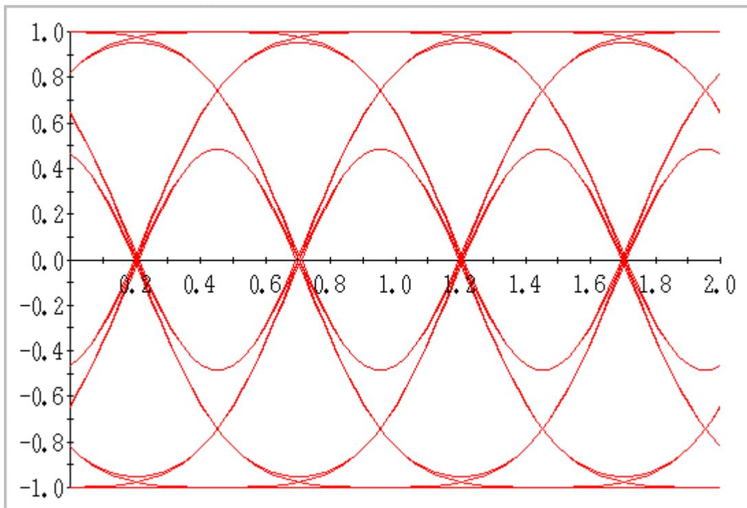
Figure 2. Four symbols of GMSK gaussian filtered phase,  $BT=0.3$ . Note the significant ISI.
