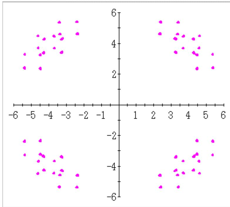
Figure 9. CQPSK receive constellation. The wide spreading of the constellation points indicates the presence of significant ISI.
