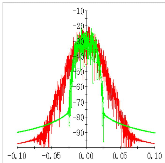
Figure 12. The modulated spectra of QPSK and CQPSK overlaid for comparison. The QPSK signal is represented by the green lines while CQPSK is indicated by the red lines. The QPSK signal was filtered with a 40% Root-Raised-Cosine Nyquist transmit filter. QPSK provides much better spectral efficiency as long as the power amplification provided by the HPA is highly linear.
