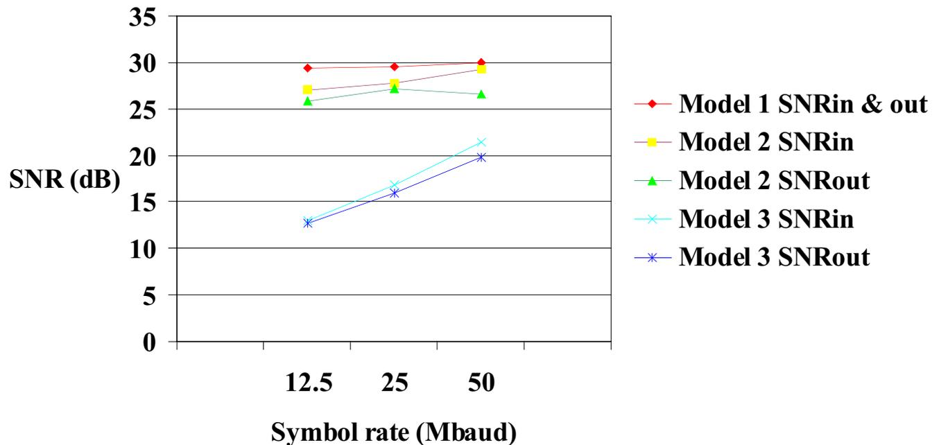
**Fig. 2** SNR at receiver input after filtering, and at fractionally-spaced DFE output for Models 1, 2 and 3
