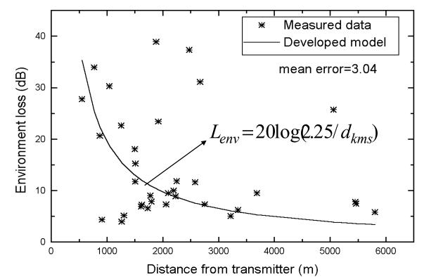
• Additional loss caused by climatic conditions, multipath and shadowing effects from surrounding buildings, foliage etc.,
