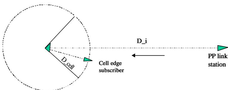
Fig. 1 Interference geometry (PP link to PMP BS)
