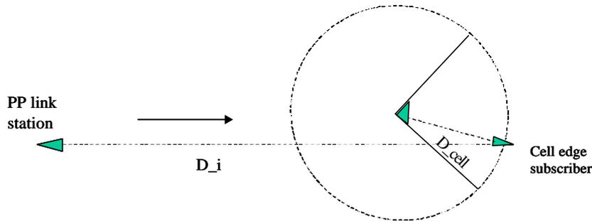
Fig. 2 Interference geometry (PP link station to PMP SS)
