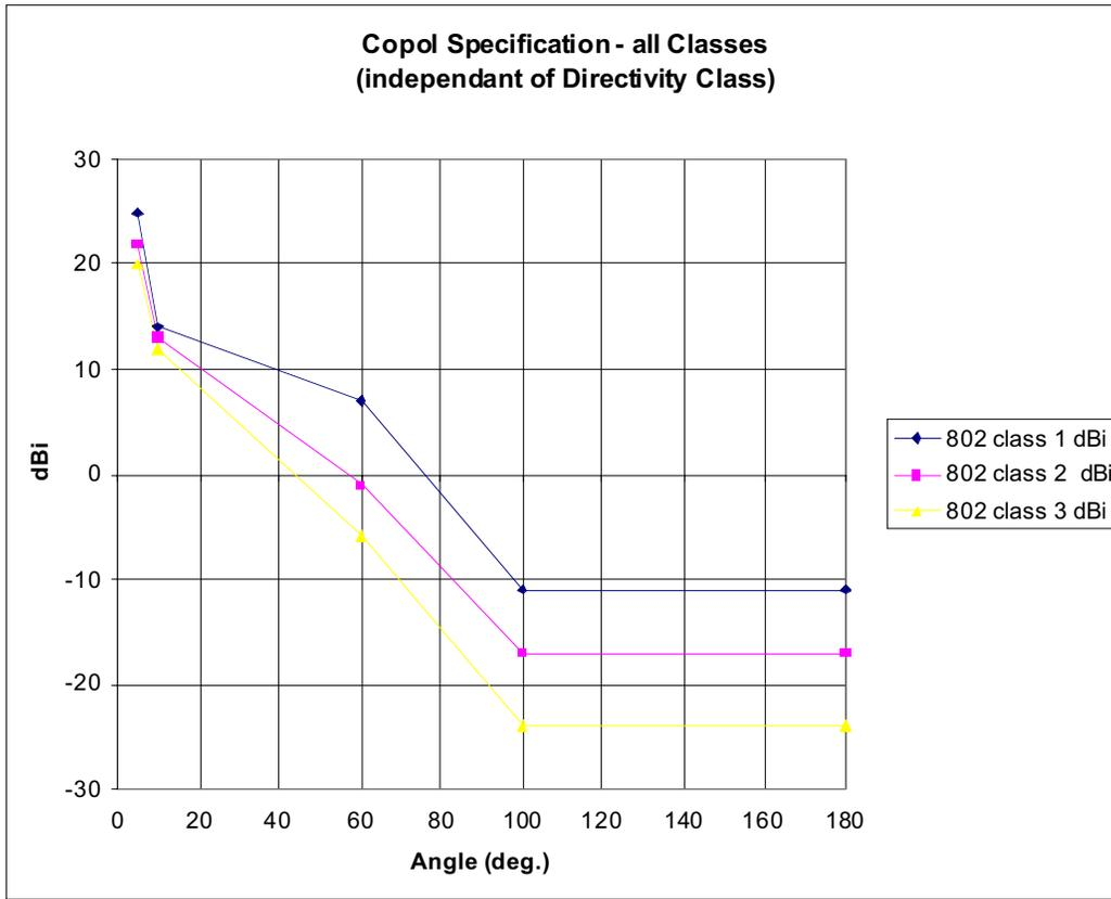
Figure 1. Azimuth RPE for Proposed IEEE TS Antennas
