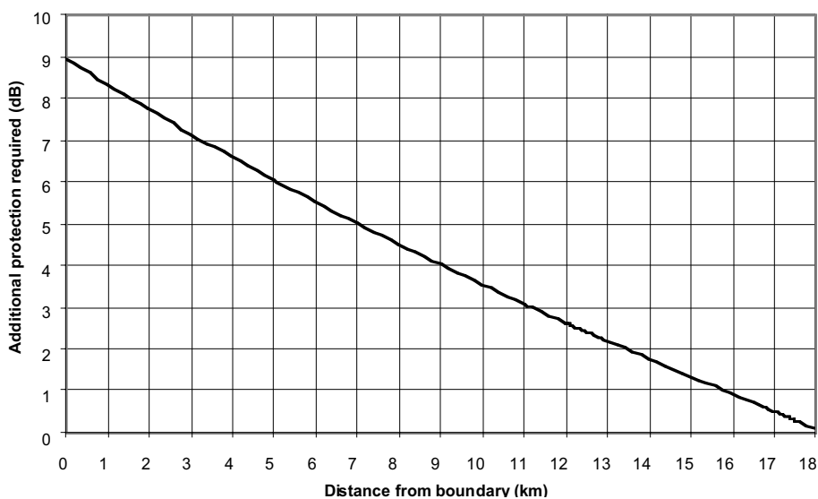
Figure A4.4 Additional shielding or off-axis discrimination required for base station as a function of distance from service area boundary (42 GHz band)
