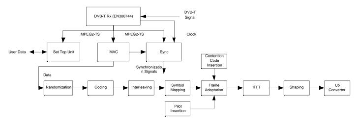
In this diagram we can notice that the user includes a simplified DVB-T receiver for the reception of the down stream. From the downs stream transmission parameters and clocks are extracted and used for the upstream creation.
