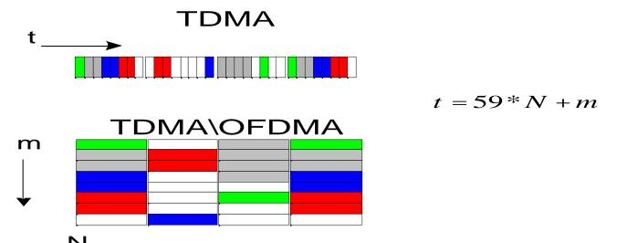
The given configuration will achieve slot granularity of ~18 bytes in QPSK with 1/2 code rate.
