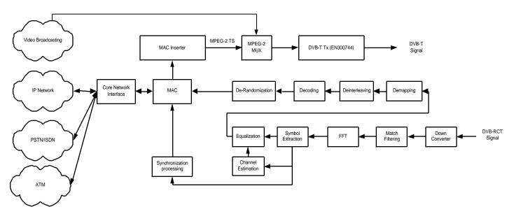
In this diagram we can see that user's Data is extracted at the Base Station and transferred by a convergence layer to the MAC. The down stream which can be composed from MAC messages or other MPEG-2 source are multiplexed into the Down Stream, the MAC messages should only be encapsulated into MPEG-2 Transport Stream, by simple means of adaptation.
