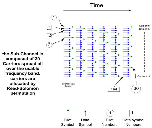
This scheme of allocation serves both frequency and time diversity. Additionally the allocation can differ to fewer carriers comprising a smaller Sub-Channel but more OFDMA symbols in time. And can be seen in the next figure:
