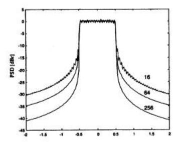
The figure illustrates the decay of the OFDM symbol when using different sizes of FFT as we can see 6dB reduction is achieved by quadrating the number of points therefore the difference between 64 points and 2048 points is about 15dB. The figure shown above is for rectangular windowing, the signal can be further perfected by adding windowing at the start and at the end of the signal, by that a DVB-T modulator can reach an 85dB decay 1/20 the frequency band away, as seen in the next figure:
