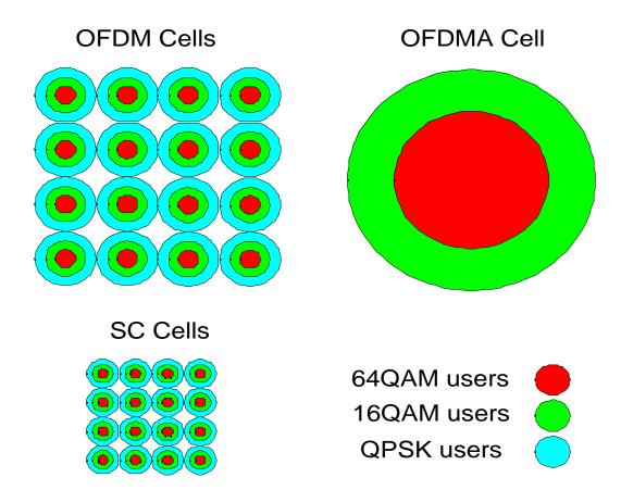
The second figure ideals with the capacity issue of cells where capacity limitations are the main problem and the OFDMA system performs better due to the use of higher constellations.
