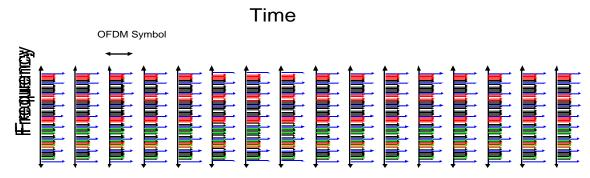
Each color in the frequency domain represents a Sub-Channel. One allocation includes allocating at least one Sub-Channel for duration of 6 OFDM symbols, this compromise is the best solution between tackling burst noise and
