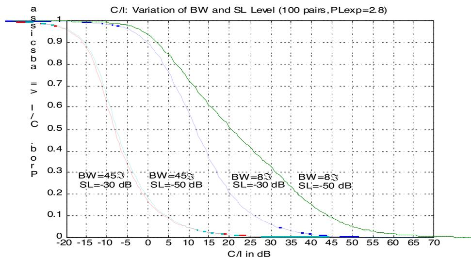
Figure 1: Probability of achieving a given C/I as a function of antenna directivity
