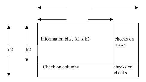
Here k1 information bits are encoded into n1 bits by using binary Hamming (n1,k1) code. This process of rowby-row encoding is applied for the first k2 rows. Hereafter, a column-by-column encoding is applied by using (n2,k2) Hamming code until all n1 by n2 matrix representing a codeword is ready.
