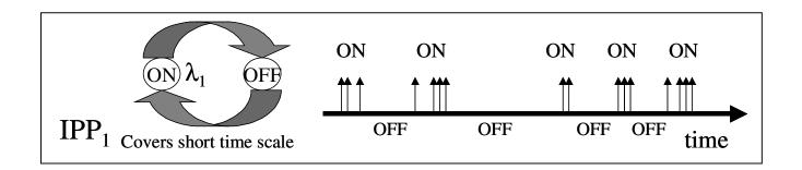
The above figure shows the packets being generated over a short time scale. The following figure shows the packets being clustered at a longer time scales. The 4IPP model superimposes 4 different time scales to generate an accurate
