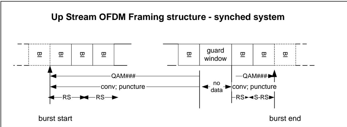
If the RF system is not synched, thus not providing orthogonality between CPE’s transmission, more than one CPE can not transmit in the same OFDM symbol. In this case any transmission of a data segment starts at the beginning of a new OFDM symbol.
