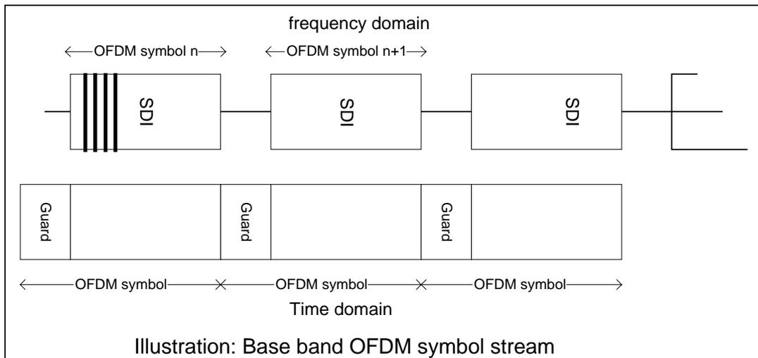
The complete process of encoding and modulation of the EOFDM signal is presented in the diagram below.
