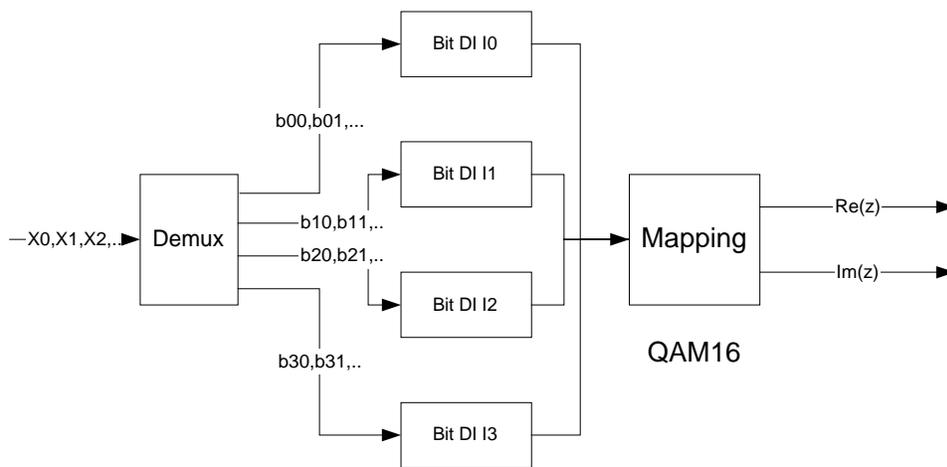
Figure 3b: Bit Di with QAM16
