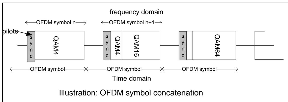
The symbol interleaving (SI) technique is applied to obtain frequency diversity. Data carrying sub-carriers are interleaved after concatenating with the sync and before the pilot insertion. The data carrying sub-carriers with different modulation level are not visually separated after the SI in the transmission, but the pilots are still placed in the fix positions. This is demonstrated in the figure below.
