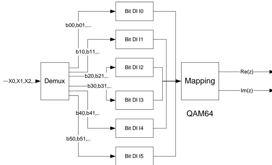
Figure 3c: Bit DI with QAM64
