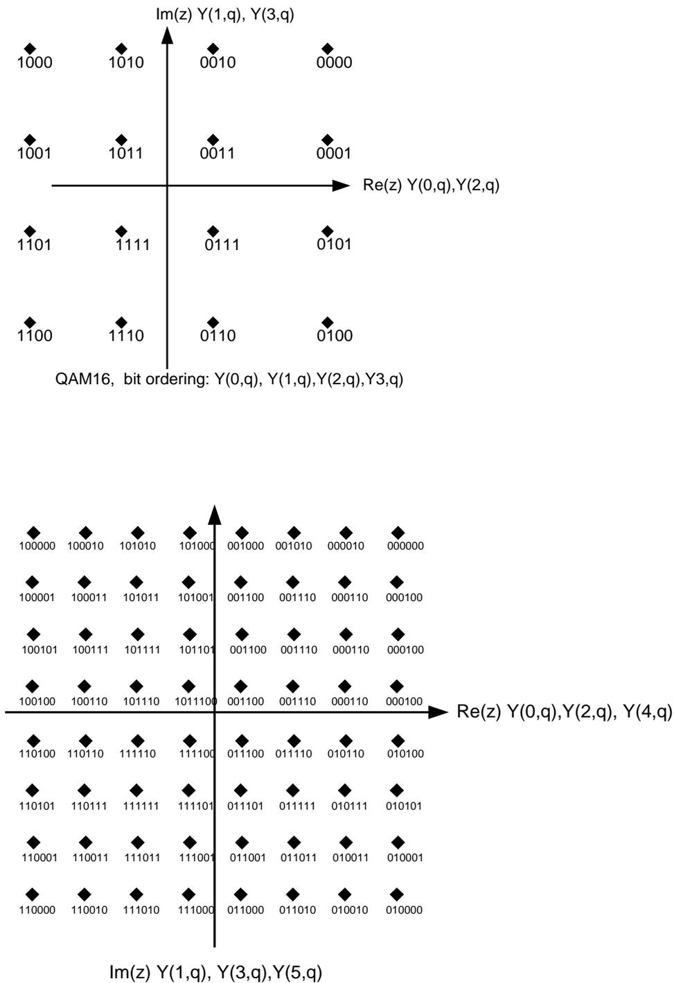
Figure 4c: QAM64, bit ordering:  $Y(0,q), Y(1,q), Y(2,q), Y(3,q), Y(4,q), Y(5,q)$
