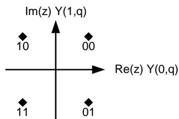
Figure 4a: QPSK, bit ordering: Y(0,q), Y(1,q)
