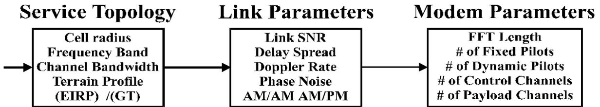
Figure 1. OFDM Design Methodology and Specification Flow
