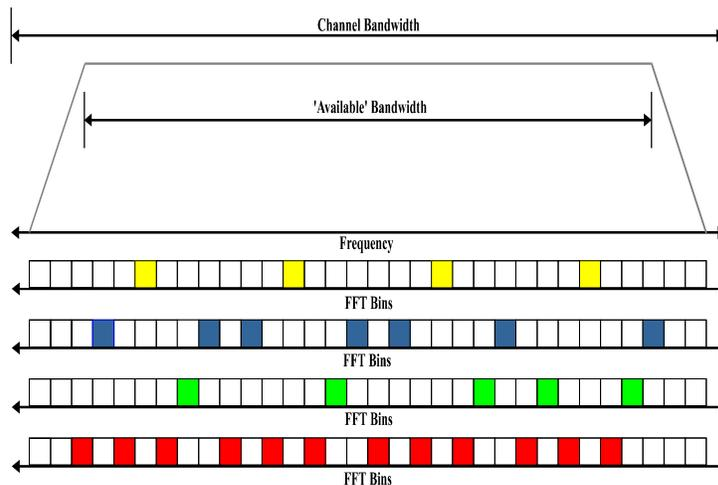
**Figure 4. FFT and Signal Channel Assignments vs. Available Channel Bandwidth**
