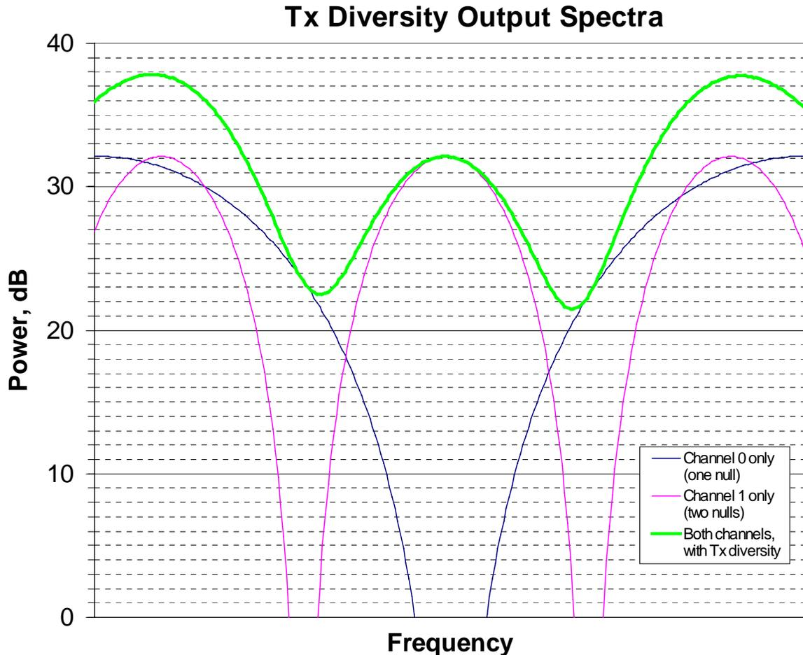
Figure 9. Transmit Diversity Output Spectra
