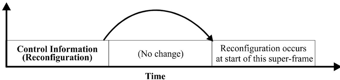
**Figure 6. Control Channel Reconfiguration Timing**
