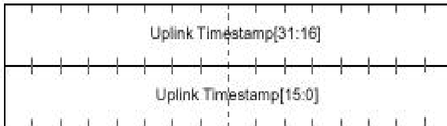
Figure 5.14: PHY Synchronization Field (PHY Type = {0,1})
