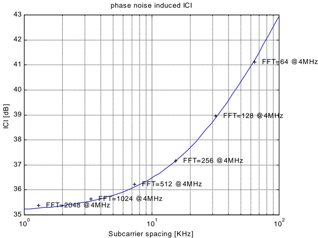
Figure 2 ICI induced SNR vs. Subcarrier spacing
