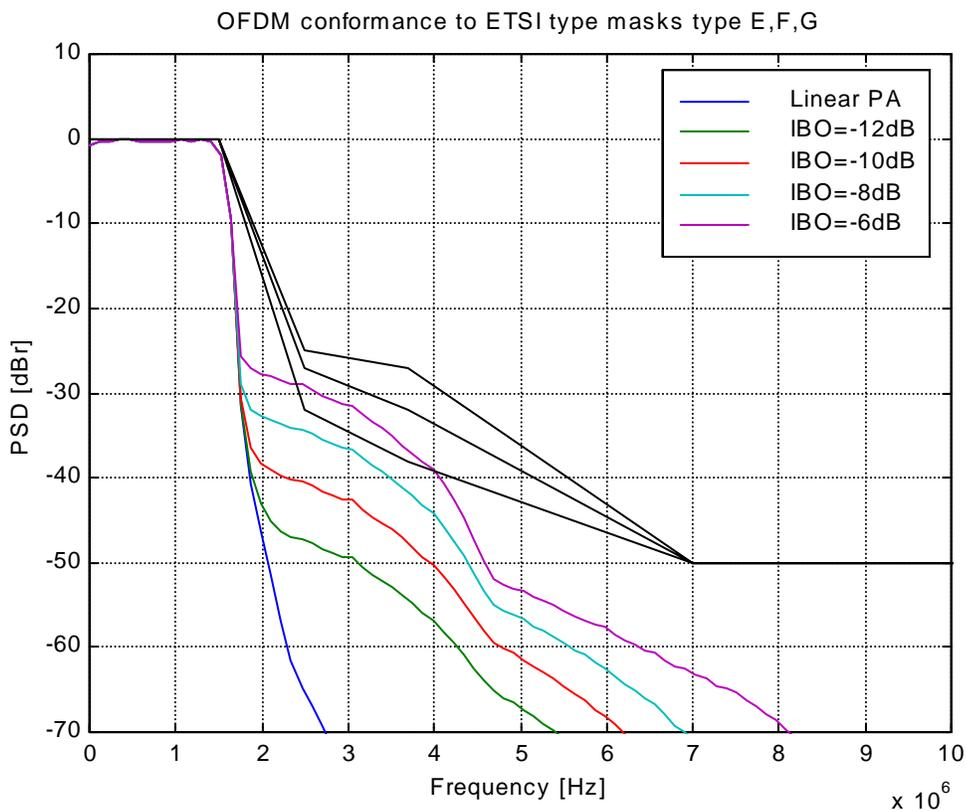
Figure 3 OFDM conformance to ETSI mask
