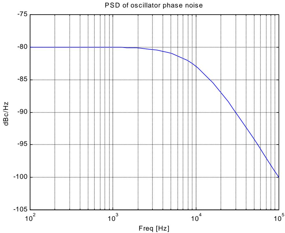
Figure 1 PSD of phase noise process
